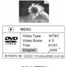
For example, to navigate to a specific chapter, press the UP/DOWN ARROW buttons to select the "Chapter" item, and then press the SELECT button.
