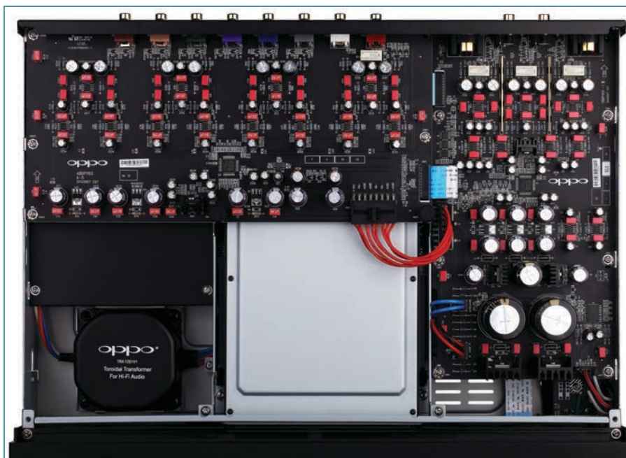
Photo 3: The BDP-105's multichannel audio board is located in the upper left. The dedicated two-channel audio board is on the right. The video circuitry and its switching power supply are fully shielded and located in the bottom portion of the player. The unit features excellent construction quality and a robust steel chassis.
